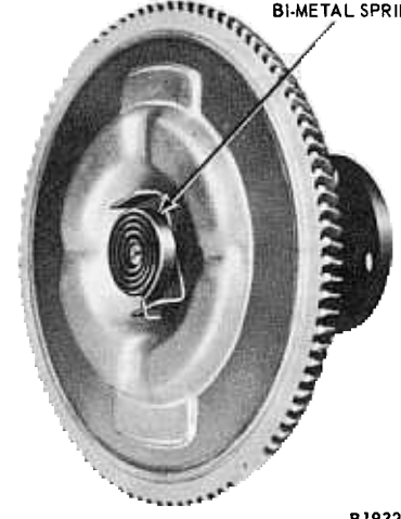
FIG. 5—Fan Drive Clutch With Flat Coil Bi-Metal Spring
